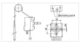
Electrical contact capacity = NC 16(6) / A 250 Vac Switches = changeover Max. head temperature = 85°C Min. capillary curvature radius = 5 mm Connection = via faston 6,3x0,8 Certifications = CE, ENEC03, EAC, UL
